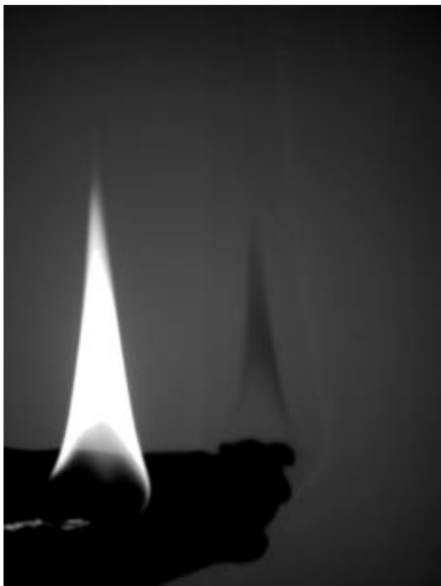
A spotlight is directed at a flame. The flame produces a shadow. The reason: soot particles.
